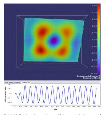
Full-field vibration of a membrane with temporal displacement of the central point.
