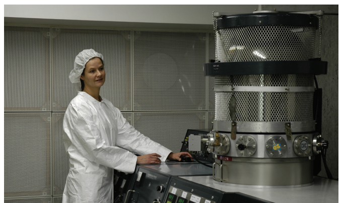
Thin film coating in Dantec Dynamics' clean room facility.
