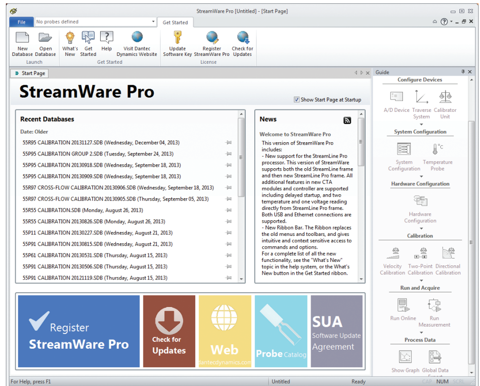
StreamWare Pro software has a modern look and an intuitive interface, which guides the user through system configuration, hardware setup, probe calibration, and data acquisition.
