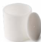
Large crucible made of Al 2 O 3 , volume 300 µl
