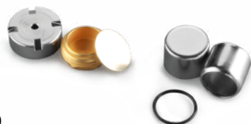
Medium-pressure crucible (right) and high-pressure crucible (left)
