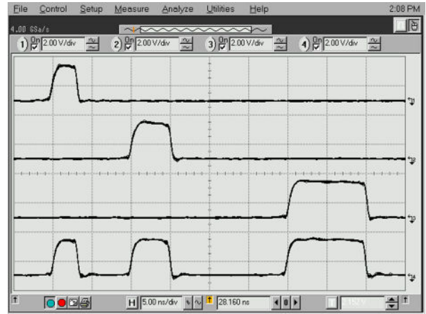
Combinatorial outputs showing 3 ns, 5 ns and 10 ns pulses with 1 ns transition times (5 ns/div)
