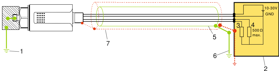
Fig. 10: Standard earthing concept
