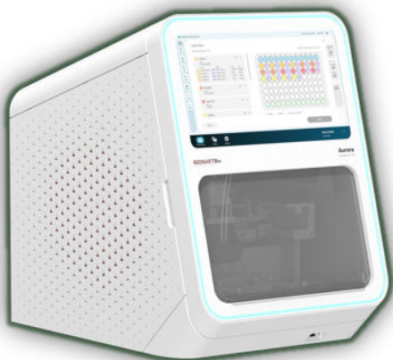
Figure 1. Aurora Tx used for structure and T_m characterization.
