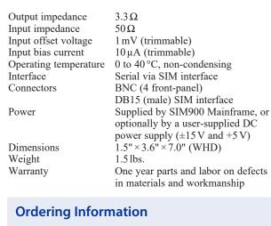
SIM954 300 MHz inverting amplifier
